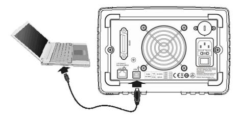
After successful connection, turn on the instrument and a dialog will pop up to guide you to install the driver of "USB Test and Measurement Device" on the PC. See figure below.
