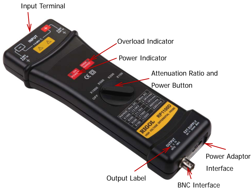
Figure 3 RP1100D High Voltage Differential Probe
