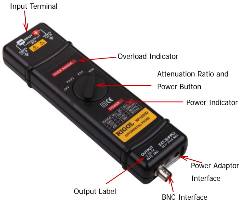
Figure 1 RP1025D High Voltage Differential Probe
