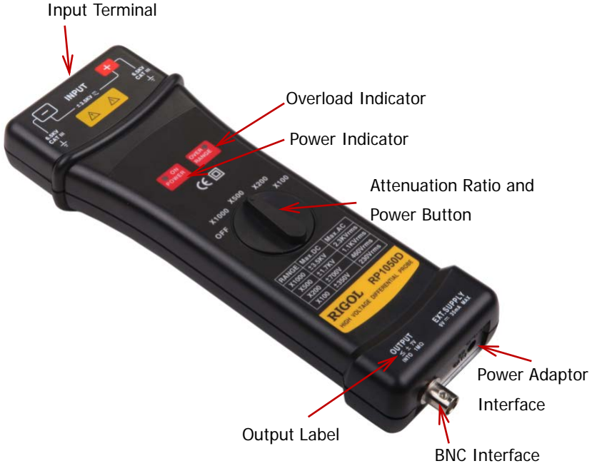
Figure 2 RP1050D High Voltage Differential Probe
